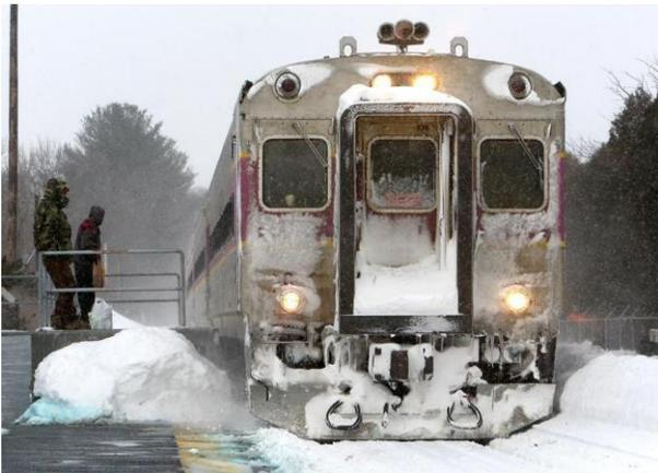
A commuter rail train arriving at North Beverly. Rail vehicles ingest snow accumulated on track areas, platforms, and switches, resulting in motor damage. Source: Boston Globe
